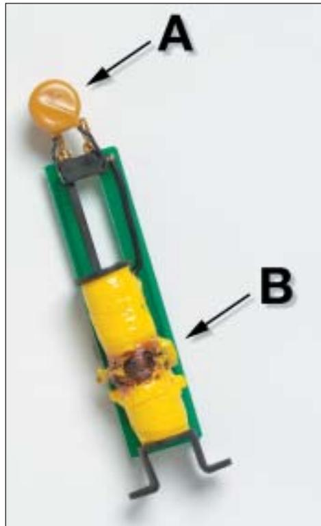
**Figure 1:** This solenoid tester experienced a catastrophic failure after receiving an impulse. Even with an MOV (metal oxide varistor) (see A), the unit will still self-destruct from overheating (see B).
