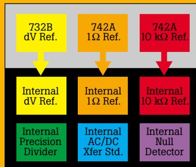
into the instrument. At that point, the calibrator measures, verifies, and adjusts itself, reducing an eight-hour job to about one hour. Thousands of 5700A calibrators in service around the world prove Artifact Calibration delivers fast, easy, and inexpensive calibration along with the confidence that your instrument is performing as expected between calibrations.
