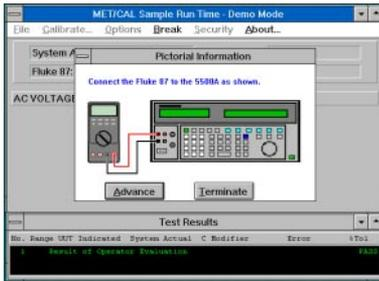
MET/CAL is a powerful environment for creating, editing, testing, and documenting calibration procedures, and for performing automated calibrations. It supports a wide variety of standards and includes more than 300 procedures.
