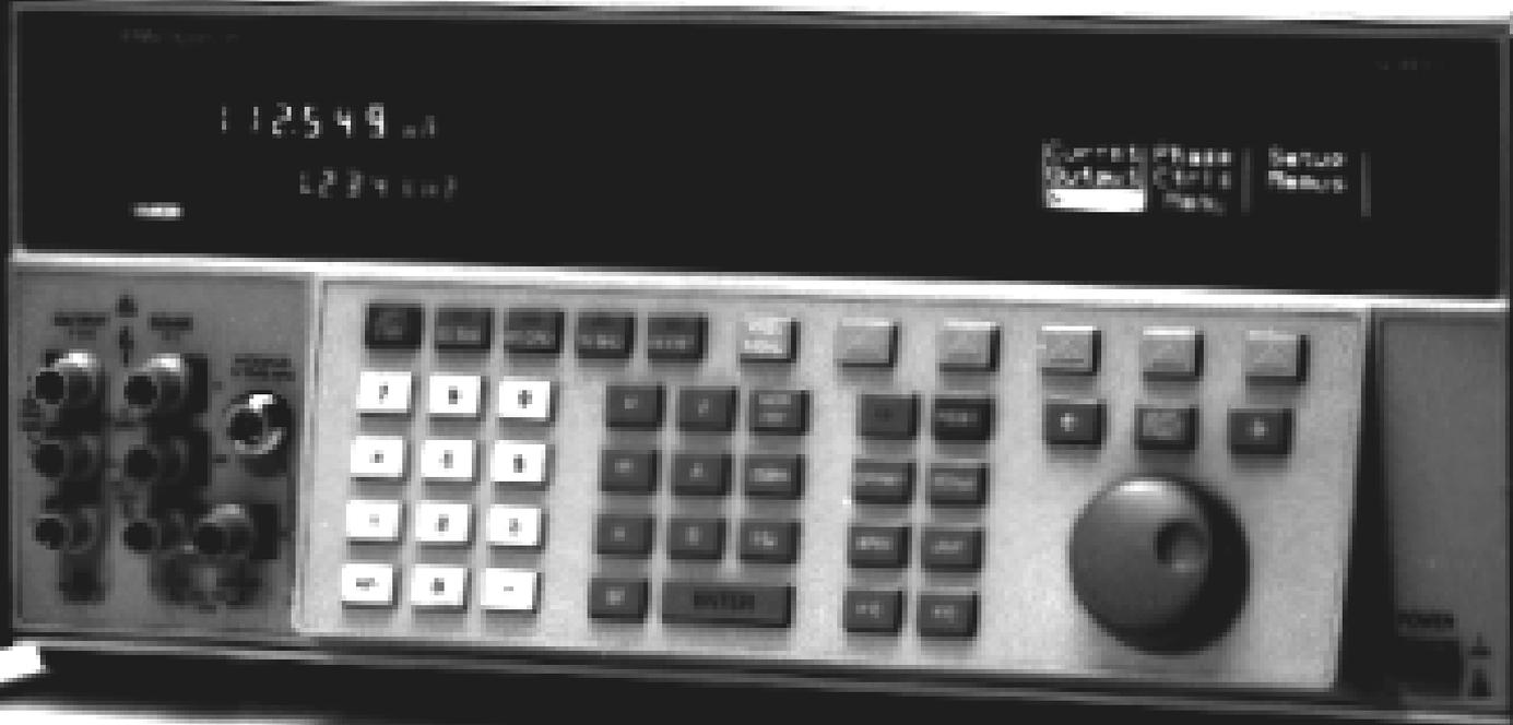
Both the 5700A Series II and the 5720A feature RS-232 and IEEE-488 interfaces, and can control Fluke 5725A, 5220A, and 5205A/5215A Amplifiers, so they are compatible with your existing equipment. Both also feature Artifact Calibration which helps keep support costs low while providing confidence that your instrument is performing as you expect it to.
