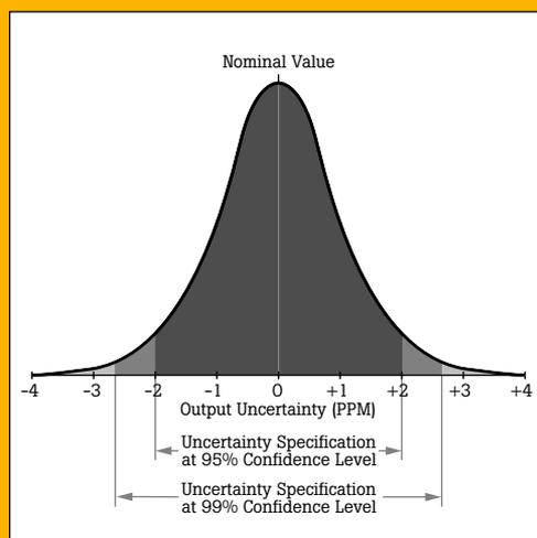
A critical factor in specified calibrator performance is the difference between the actual output value and the nominal output value. The confidence interval is a statistical expression of the likelihood that any output of any instrument will deviate beyond this specified difference or uncertainty.
