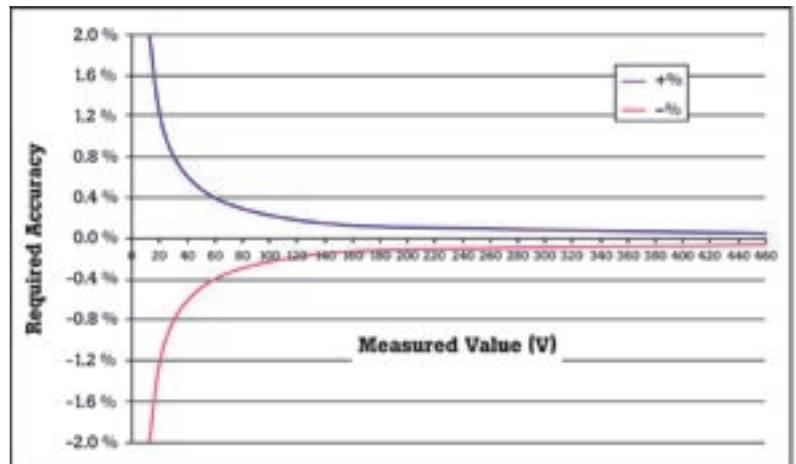
Figure 1: This graph illustrates how .1 % of declared input voltage uncertainty impacts the accuracy of a measured voltage. Note how at 230 V the uncertainty is 0.1 %.
