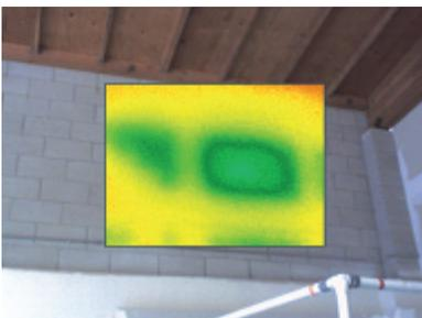
Figure 4: IR-Fusion helps pinpoint problems in buildings by combining infrared and visible images.
